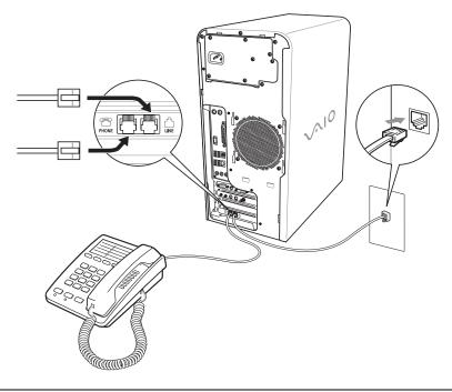
Your computer has a protective sticker 😿 covering the Ethernet port located on the rear panel. Connect only 10BASE-T and 100BASE-TX cables to the Ethernet port. Using other cables or a telephone cable may result in an electric current overload that can cause a malfunction, excessive heat, or fire in the Ethernet port. For help on connecting to a network, see your network administrator.
